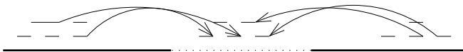
Fig. 7. Gaps in scaffolds can be filled by re-mapping the reads onto the contigs.
